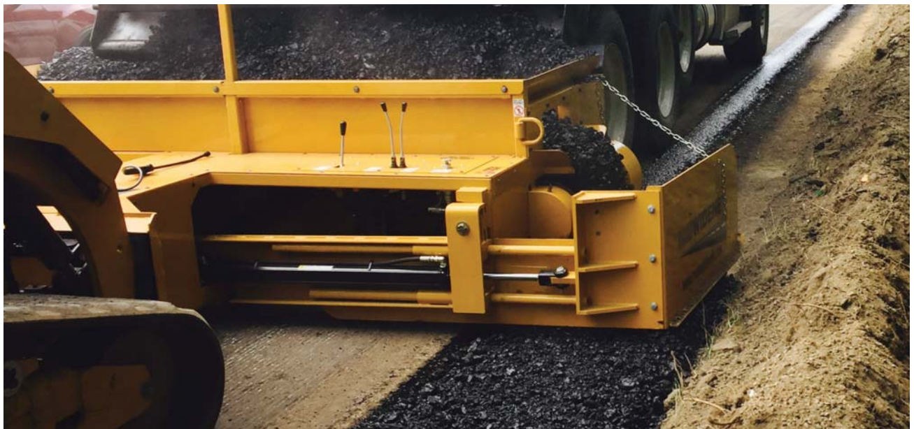
All attachments are equipped with a heat-treated belt, creating a versatile machine that can lay down any material, including hot mixes.
